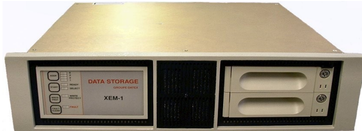
Dual Rack Mount XEM1 A/B with Tape Backup (L) and Disk to Disk Copy (R)
